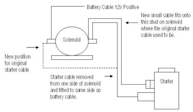
Since the Hi-Torque starter has it's own solenoid fitted you need to make a couple of changes.
